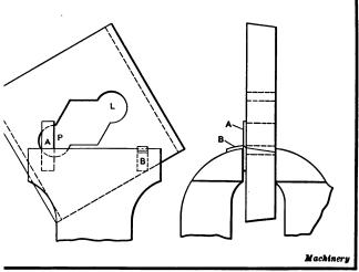
Fig. 15. Blanking Die in Vise ready for Filing
